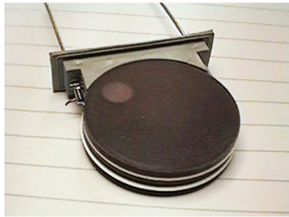
Figure 6. Photograph of a partially dismantled polypropylene case tantalum Hybrid capacitor showing stacked arrangement of anode electrodes connected in parallel. The top cathode plate and separator has been removed .
