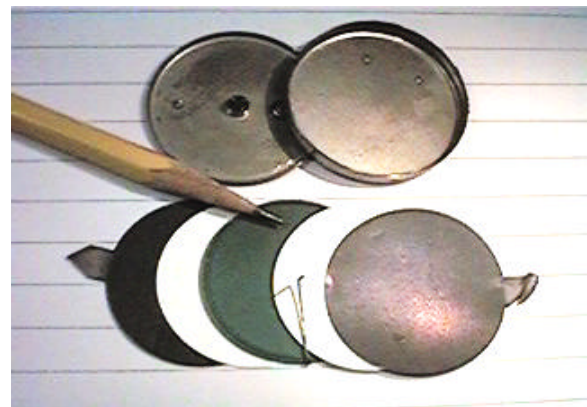
Figure 3. Photograph of a dismantled tantalum Hybrid capacitor showing anode, cathode, and case elements.
