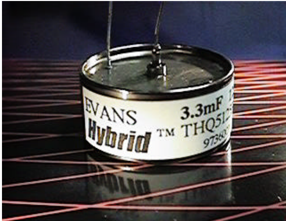
Figure 1. Photograph of a 125 V, 3300mF hermetic tantalum Hybrid capacitor.
